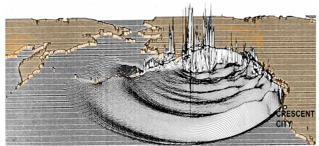
Snapshot from a numerical model of the 1964 tsunami at about three hours after the earthquake. This was roughly the time Del Nort County was first notified that a tsunami could be on its way. Vertical scale is highly exaggerated.
