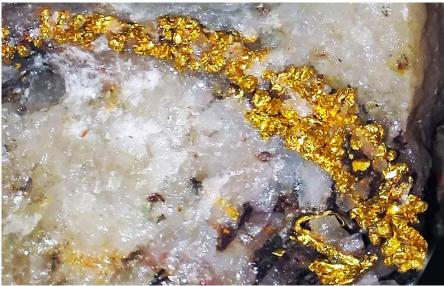
Concentrations of gold in quartz like this sample from the Red Mountain Mining District near Ouray, Colorado may be the caused by repeated earthquakes.
